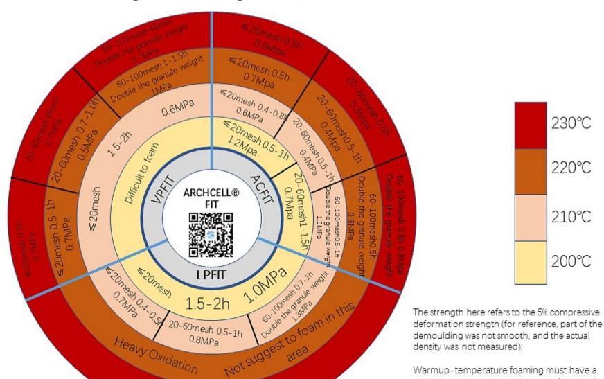
temperature-warmup process, and cannot be directly placed in a high-temperature oven, otherwise small particle will not be fully
